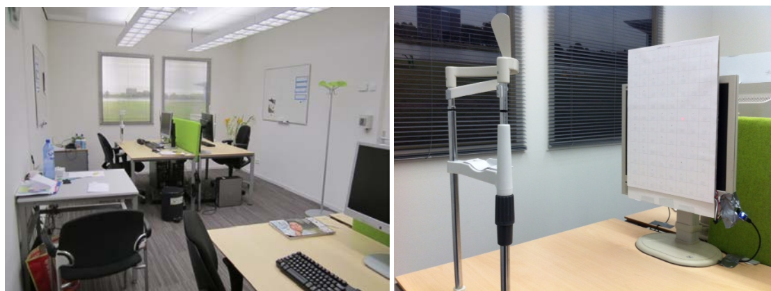
Figure 1 – Left: Photograph of the simulated office room in which four participants were seated at a desk in front of a monitor. The desk on the left was used by the test leader. Two artificial windows are visible in the rear wall. Right: Photograph of the paper-based Landolt-C visual acuity test set-up used.
